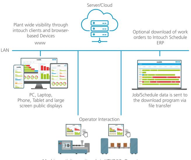
Machine activity monitored via XTX7/15. Operator access to Intouch system also via XTX7/15 HMI.
