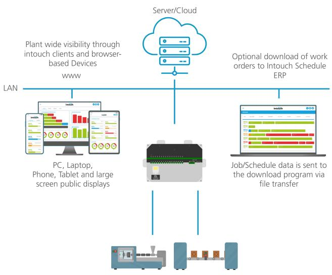
Machine activity monitored via XTX016C. Operator access to Intouch system via third party device.
